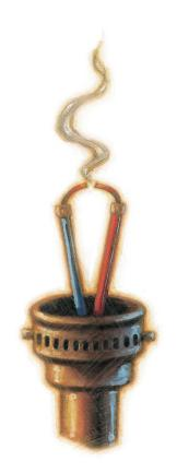
Instead of using a very thin piece of paper, he used a threadlike piece of cardboard. Thomas boiled it with certain chemicals, and then baked it until it became coated with carbon. He used this filament in a new bulb without air.
